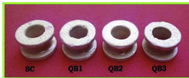
Fig. 2. Standard and experimental ceramic insulator.
